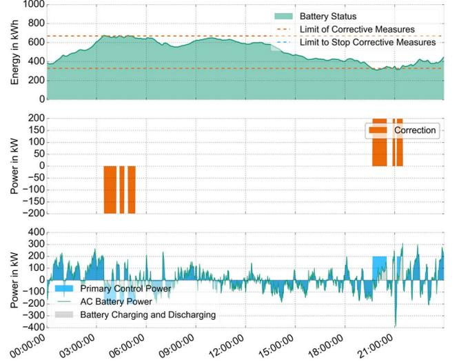
Figure 2 Exemplary Operation of a BESS with 1-C providing FCR with 80 % of the nominal power with 30 minutes minimum activation period and *Corr* method to calculate the limits of corrective measures.
